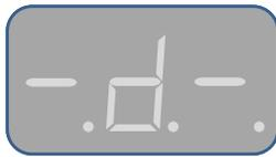
Abb. 13: Display Magneta D Smedegaard - Symbol Firmwaretest
